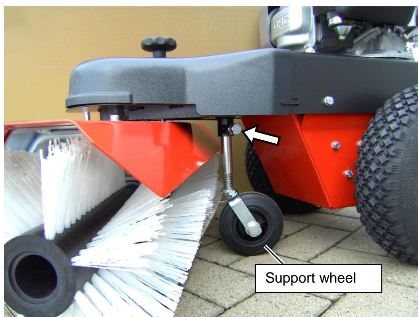
Fig. 7: Support wheel with clamp screw (arrow)
