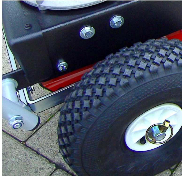
Fig. 6: Correct installation – steering arm / support bracket
